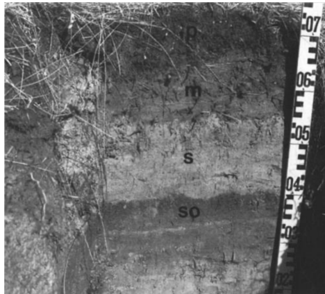
Alternating layers in a pit near Tofino, BC: Soily peat (so), sand (s), mud (m), and peat (p) J.J. Clague, 1997.
