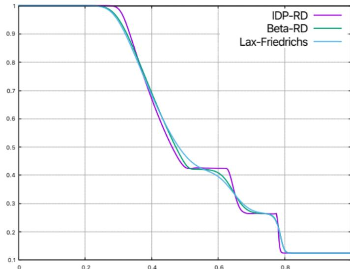
Figure: Sod shock tube test, 200 cells, quadratic Bernstein polynomials
