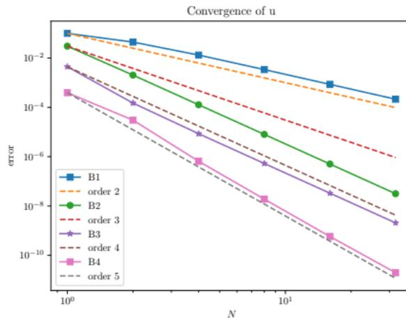
Figure: Convergence analysis for pure diffusion with RD solver.
