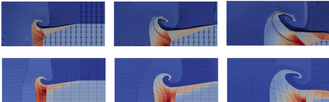
Figure: Density (cell averages) at  $t = 2, 3$  and  $4.3$  for Triple Point problem. **Top:** Q1Q0 solution with  $\sim 173\text{k}$  nodes. **Bottom:** Q4Q3 solution with  $\sim 12\text{k}$  nodes.
