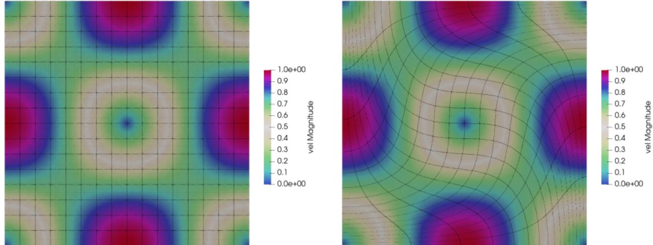
**Figure:** Q4Q3 simulation of the Taylor-Green Vortex. The mesh is  $16 \times 16 \times 1$ . The velocity field is shown at  $t = 0.0$  (left) and  $t = 0.5$  (right).
