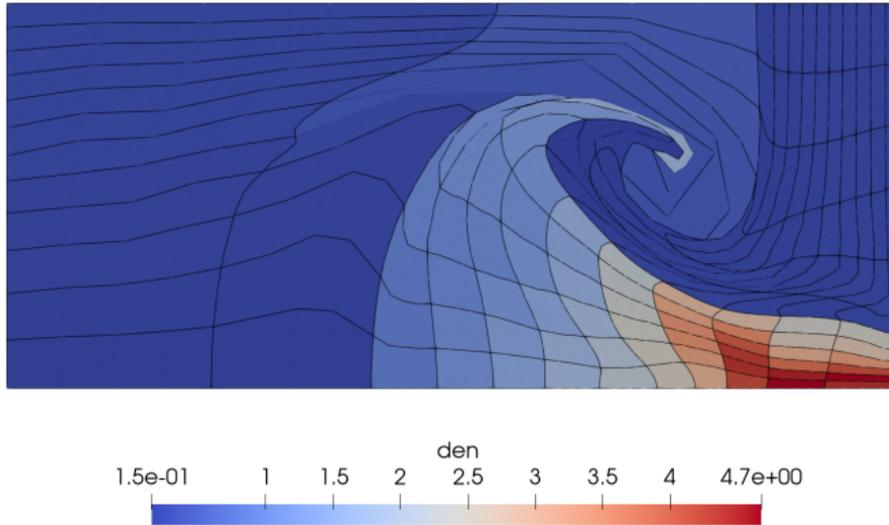
**Figure:** Q4Q3 simulation of the Triple Point problem. The mesh is  $12 \times 12 \times 1$ . The cell-average density is shown at  $t = 5.0$ .
