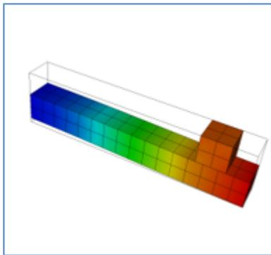
Finite deformation implicit mortar contact
