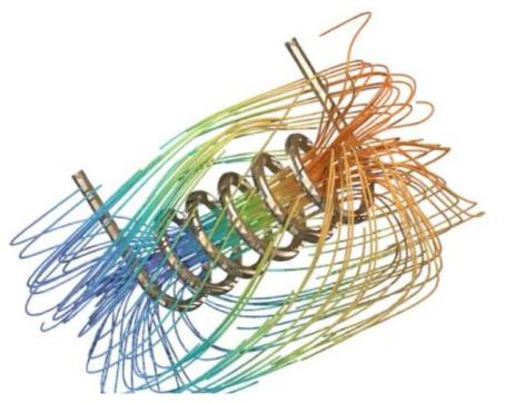
Magnetic diffusion problem solved to compute the magnetic field induced by current running through copper wire in air. The problem is solved using the A-phi formulation, using GPU-accelerated low-order-refined solvers in H1 and H(curl). The magnetic field is represented as a Raviart-Thomas finite element vector field in H(div).
