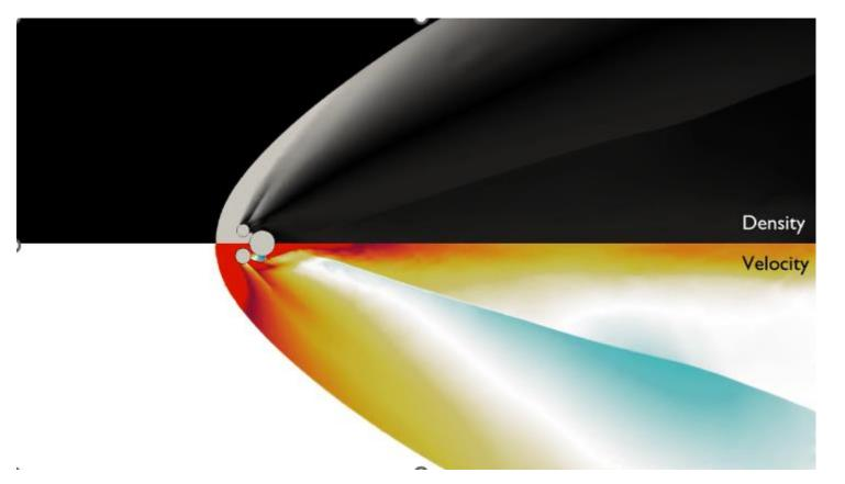
Tim Brewer Synthetik Applied Technologies Single phase compressible Euler simulation using a DG discretization to describe supersonic (Mach 2.5) flow around cylindrical obstructions. The simulation leverages Synthetik's newly developed code for highly compressible flows.
