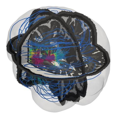
Streamlines of the electric field generated by a current dipole source located in the temporal lobe of an epilepsy patient. Finite element solution using a regular hexahedral grid implemented in MFEM. Visualization with ParaView.
