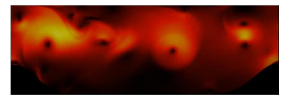
Turbulent Incompressible Navier-Stokes LES flow through a periodic hill, H1 p=4, Re=5000
