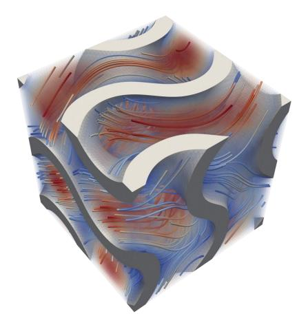
Flow through periodic Gyroid micro-cell, MFEM Navier miniapp with additional Brinkman penalization
